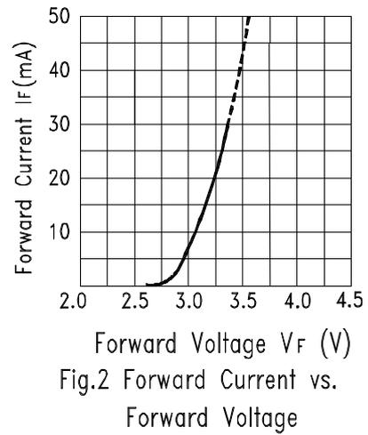
Fig.2 Forward Current vs. Forward Voltage
